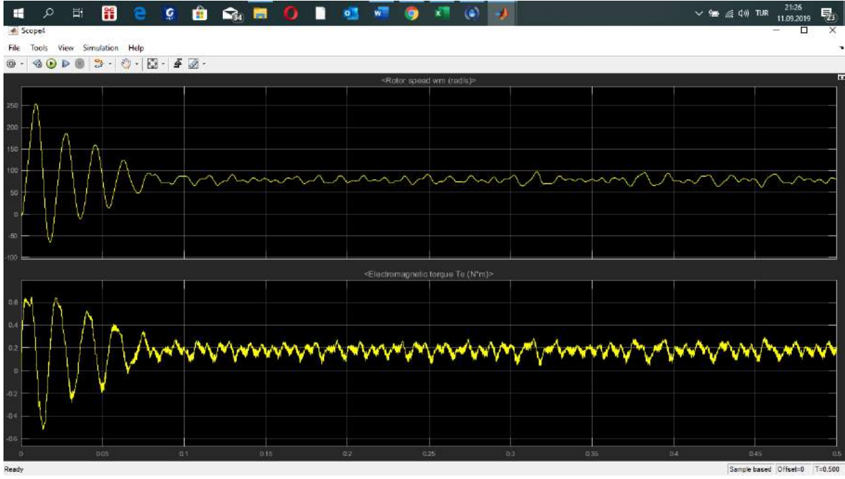
Fig.13 Electromagnetic torque and speed representation between [0 – 0.5] second when R_s=0.55 \Omega
