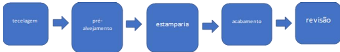
Figure 2. Fabric production flow steps. Source: The author.
