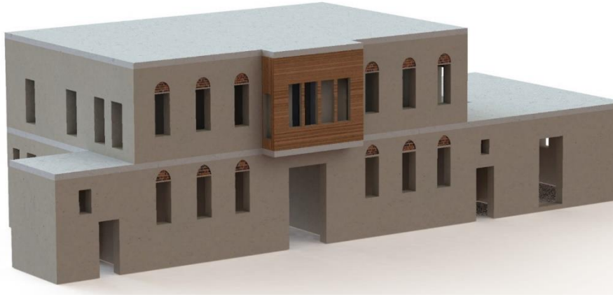
Fig. 5. Finite element model of the building
