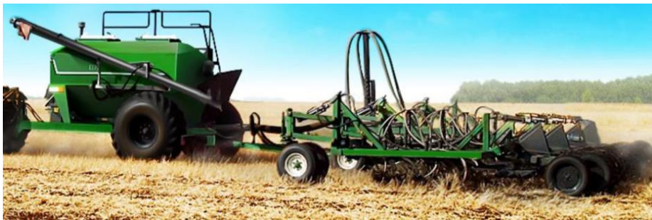
Figure 4 - The sowing complex (SC) "Kuzbass"
