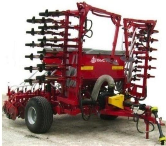
Figure 1 - Universal pneumatic seeder grain-fertilizer C - 6PM.1
